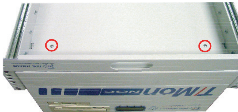
Fig. 1.1 - These screws secure the T/Mon NOC to the Slide Rack
