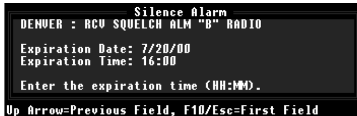
Fig. 16.21 - Silence/alarms windows allows a nuisance alarm to be suspended for a limited time.
