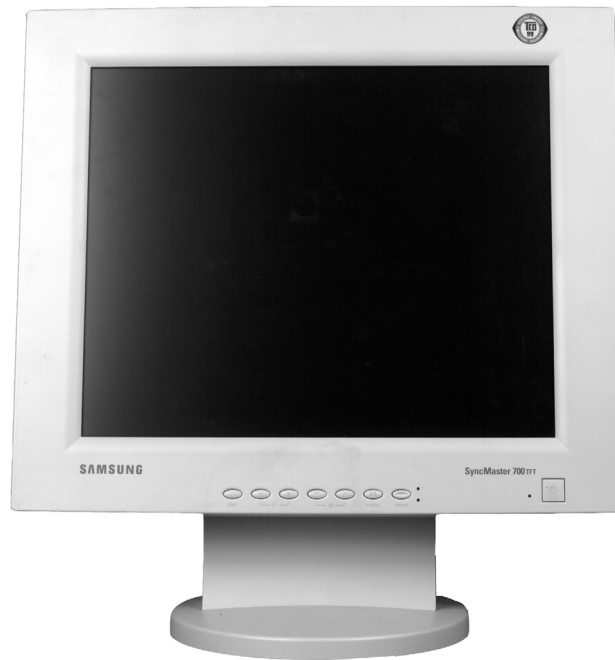
Fig. M.31 - Monitor controls are located on the front of the unit
