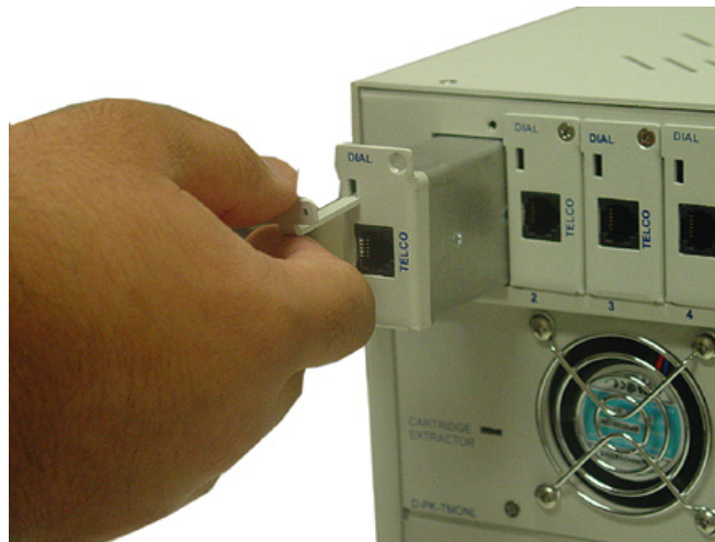
Fig. 1.15 - Use the Cartridge Extractor to remove the old Port Interface Cartridge
