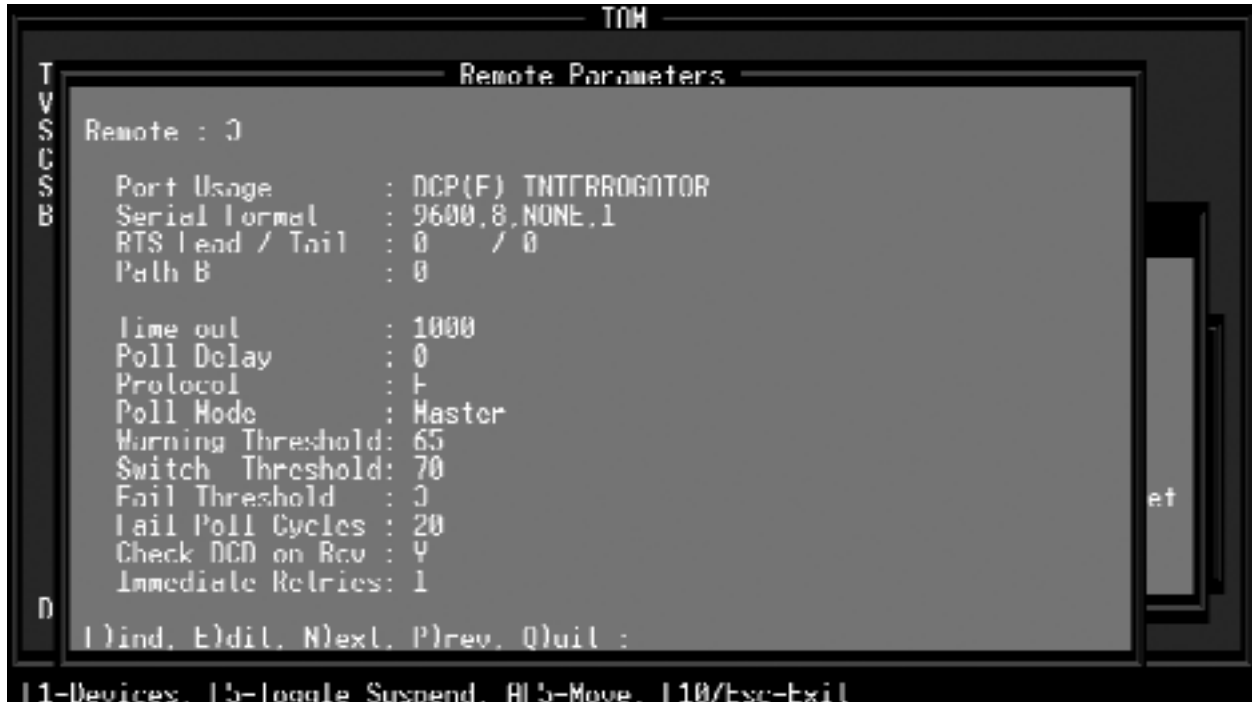
Fig. M1.45 - Set data rate to 9600 baud and DCD on for protection switch port.
