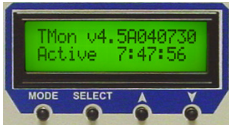
Fig. 1.18 - The T/Mon NOC LCD display, showing the Standard Prompt
