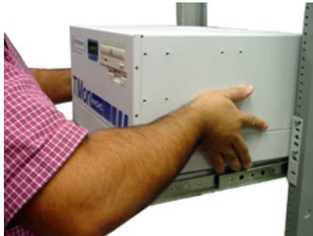
Fig. 1.3 - Place the T/Mon NOC on the extended Slide Rack
