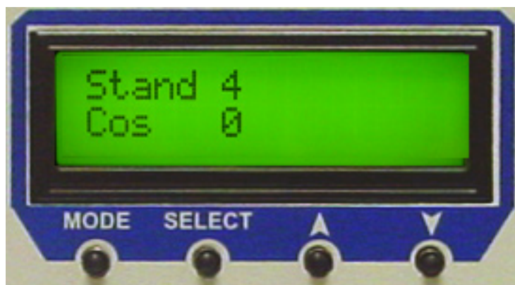
Fig. 1.19 - Standing/COS Alarm Display
