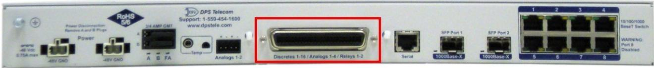
*Alarm and control relay connectors*
