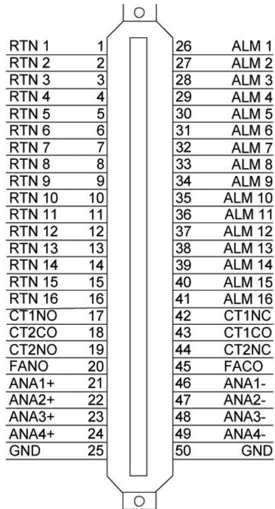
*Pinout Diagram for Discretes 1-16 connector*
