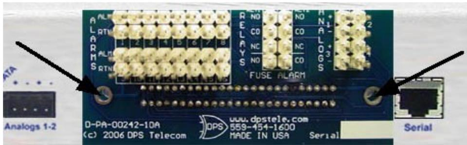
*The wire-wrap back panel (arrows indicate screw locations for mounting)*
