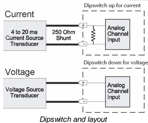
The analogs are controlled by the dipswitches to the left of the Amphenol connector (located at the back of the unit). For milliamp sensor operation, turn the dipswitch on by placing it in the on position. For normal operation, place the dipswitch in the off position. Note that the dipswitch is internal, and requires the case to be opened in order to change the setting.
