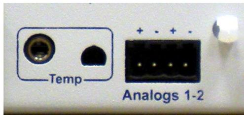
*Temperature Sensor and Analog Connectors*
