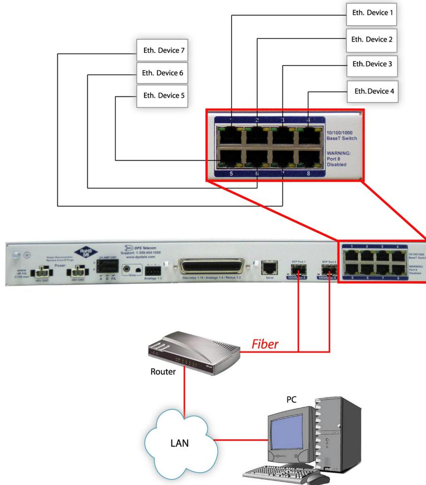
*Chart of Ethernet and SFP Fiber Interface Connections*
