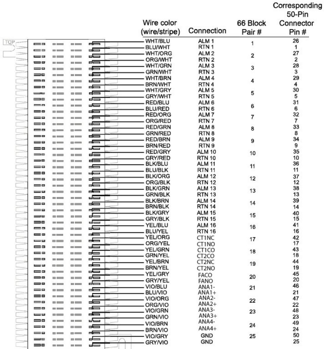
Optional 66 block pinout for Discretes 1–16
