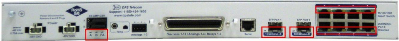
*Back panel LEDs for Power and Ethernet connections*
