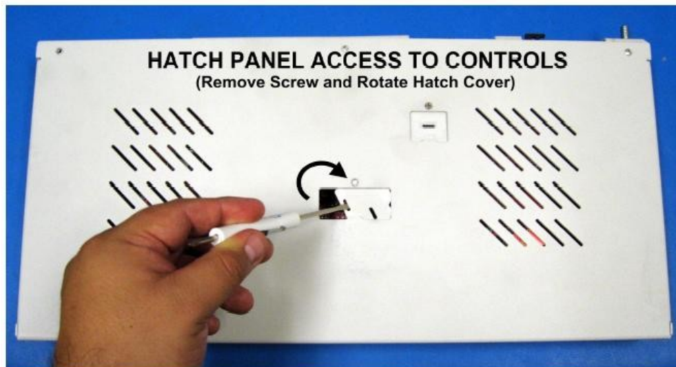
Hatch Panel Access on Top of NetGuardian G5 Chassis
