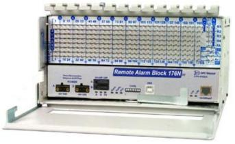
The Remote Alarm Block 176 G2 is a compact, high-capacity alarm collection remote. With 176 discrete alarms and 4 relay outputs, the RAB 176 G2 is the optimum combination of high-density monitoring in a compact form.
