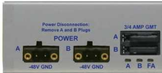
RAB G2 Power Terminals and Fuses
